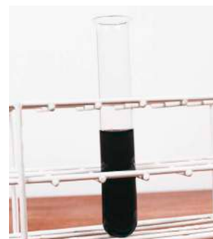
Figure 3: A starch test for iodine. Starch solution is added and the solution turns black if iodine is present.
