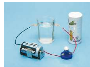
Figure 6: An experiment to test the conductivity of a solution.
