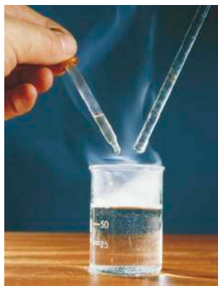
Figure 1: The reaction of an acyl chloride with water. You can see the misty fumes of \text{HCl} that are being given off.
