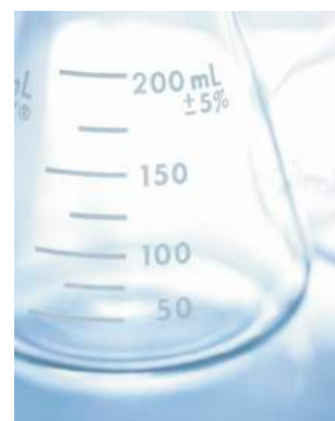
Figure 1: A conical flask where the graduations have an uncertainty of \pm 5\% .
