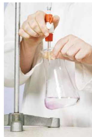
Figure 4: A titration where an alkali is being added to an acid. The indicator in the flask is phenolphthalein, so the solution starts clear and turns pink at the endpoint.
