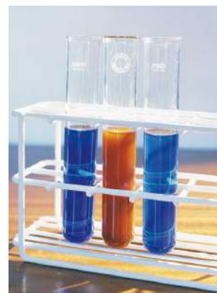
Figure 2: From left to right, these test tubes show: Fehling's solution, the brick-red precipitate made by reacting Fehling's solution with an aldehyde, and the result of reacting Fehling's solution with a ketone (i.e. no change).
