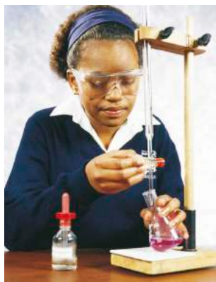
Figure 2: A student doing a titration. She is adding acid from the burette to the alkali in the flask. The alkali looks pink because it contains phenolphthalein.
