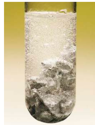
Figure 1: Zinc dissolving in hydrochloric acid.
