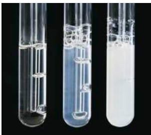
Figure 4: Limewater turns from clear to cloudy when carbon dioxide is bubbled through it.
