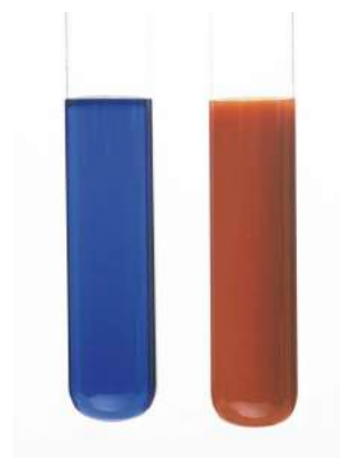
Figure 6: Fehling's solution. The test-tube on the left shows the unreacted Fehling's solution. The test-tube on the right shows the result of the reaction of Fehling's solution with an aldehyde.
