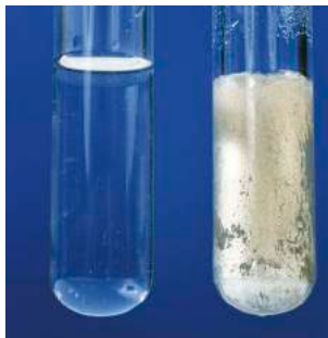
Figure 3: The test-tube on the left contains unreacted Tollens' reagent. The one on the right shows the result of its reaction with an aldehyde.
