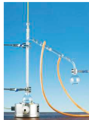
Figure 4: Laboratory fractional distillation apparatus.
