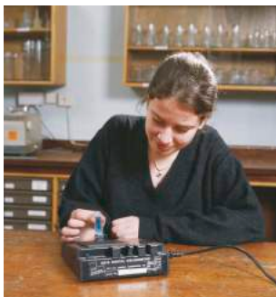
Figure 4: A student using a colorimeter to measure the absorbance of a solution of \text{Cu}^{2+} ions.
