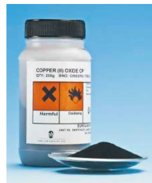
Figure 8: A bottle of copper(II) oxide. The Roman numerals show that the copper has an oxidation number of +2 .
