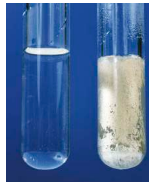
Figure 2: Tollens' reagent. The test tube on the left shows the unreacted Tollens' reagent. The test tube on the right shows the result of a reaction of Tollens' reagent with an aldehyde.
