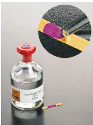
Figure 2: Concentrated H_2SO_4 is a strong acid. It turns this universal indicator paper purple, which shows it has a pH between 0 and 1.
