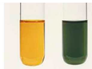
Figure 2: Alcohol oxidation. The acidified potassium dichromate(VI) ion turns from orange to green when it oxidises an alcohol.
