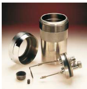
Figure 3: A bomb calorimeter. This is a very accurate piece of equipment that works on the same principle as the one shown in the diagram in Figure 2.
