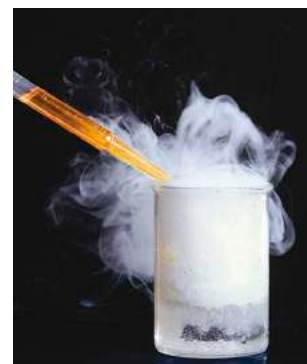
Figure 3: The reaction of an amine (the orange liquid in the pipette) with an acyl chloride, to produce an amide and hydrogen chloride gas.
