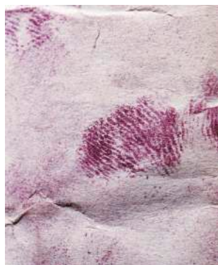
Figure 5: Ninhydrin can also be used to detect fingerprints as it reacts with the amino acids in the fingerprint, turning them purple and making the print visible.
