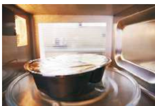
Figure 7: The containers that microwave meals come in are made of Terylene™.
