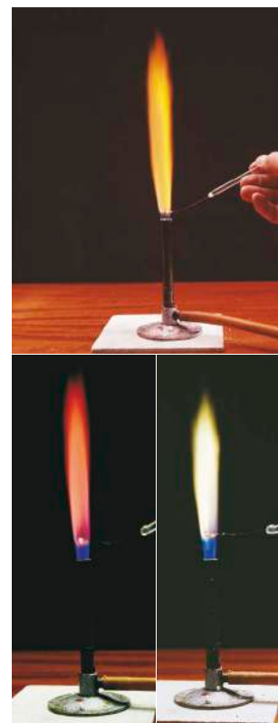
Figure 1b: Results of flame tests for solutions containing calcium (top), strontium (bottom left) and barium (bottom right).
