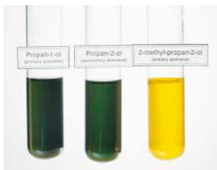
Figure 1: With a primary or secondary alcohol, the colour changes from orange to green as Cr(VI) changes to Cr(III). With a tertiary alcohol there is no reaction, so it stays orange.
