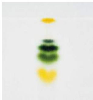
Figure 2: A TLC chromatogram.
