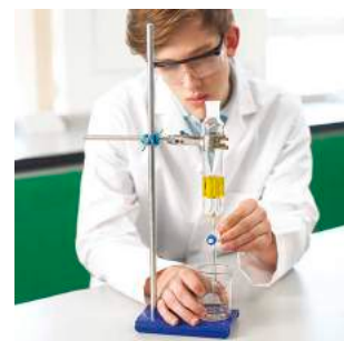
Figure 2: A student using a separating funnel to separate an organic and an aqueous layer.
