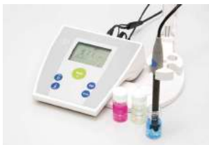
Figure 2: A pH meter is an electronic probe that you can use to accurately measure pH.
