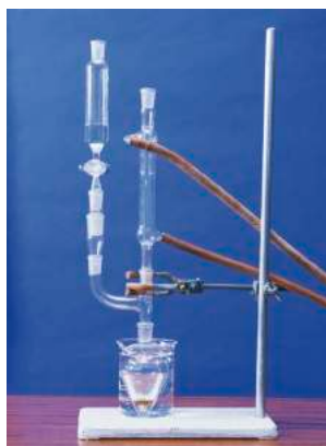
Figure 5: The reflux equipment used to make phenylamine.
