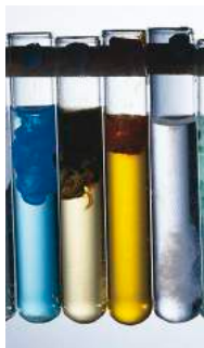
Figure 1: Metal-aqua ion precipitates. From left to right — copper(II) hydroxide, iron(II) hydroxide, iron(III) hydroxide, and aluminium(III) hydroxide.
