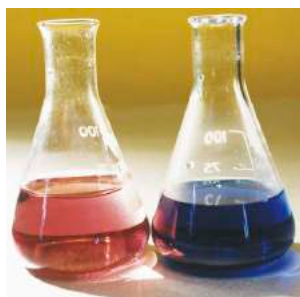
Figure 2: The flask on the left shows the pink colour of hexaaqua cobalt(II) ions. The flask on the right shows the blue colour of cobalt(II) ions complexed as [\text{CoCl}_4]^{2-} .
