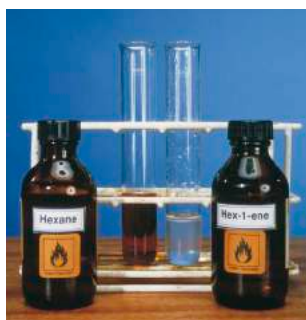
Figure 1: Bromine water test. The test tube on the right contains hex-1-ene, a compound with a \text{C}=\text{C} that has reacted with the bromine water. The one on the left contains hexane, a saturated substance that doesn't react with bromine water.
