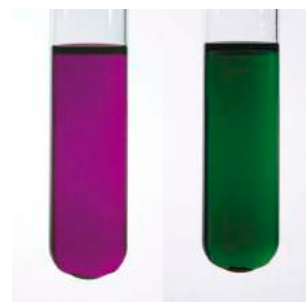
Figure 3: The test tube on the left shows the violet colour of a V(II) solution. The test tube on the right shows the green colour of a V(III) solution.
