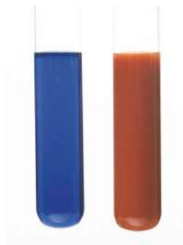
Figure 3: Fehling's solution. The test-tube on the left shows the unreacted Fehling's solution. The test tube on the right shows the result of the reaction of Fehling's solution with an aldehyde.
