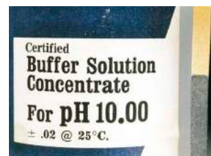
Figure 2: This basic buffer will maintain a pH of 10.00 when small amounts of acid or alkali are added.
