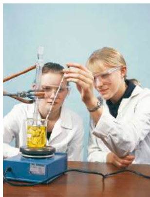
Figure 1: Two students carrying out an organic reaction under reflux, to stop the vapour escaping from the reaction mixture.
